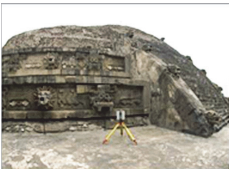
Above: Scanning by bouncing lasers off the surface on an ancient architectural structure; the sculptured Serpent Heads of the pyramids of Quetzalcoatl, Teotihuacan, Mexico. Image © Cy-Ark
